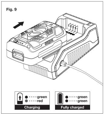
**NOTE:** If the top light remains green while the bottom light alternately flashes red and green, this indicates a temperature abnormality (i.e. that the battery pack is either too hot or too cold). If there is only a red blinking light, this indicates that something is wrong with the battery. Contact Snow Joe<sup>®</sup> + Sun Joe<sup>®</sup> customer service center at 1-866-SNOW-JOE (1-866-766-9563) for assistance.
