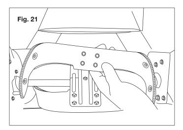
**2.** Install the new rubber plate assembly by tightening the 8 sets of nuts and bolts on both sides (Fig. 20).
