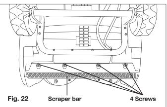
2. Detach the worn scraper bar from the snow blower by removing the 4 screws that hold it in place (Fig. 23).
