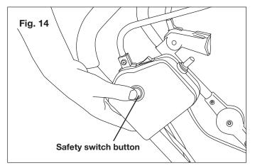
**4.** While depressing the safety switch button, pull the ON/OFF switch lever toward you. Once the machine powers on, release the safety switch button and begin operation (Fig. 15). The machine can only be started by depressing the safety switch button first, followed by squeezing the ON/OFF switch lever; reverse operation will not start the machine.
