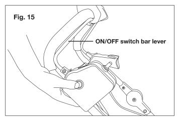
5. To power off, release your grip on the ON/OFF switch bar lever.
