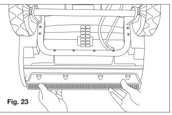
**3.** Install the new scraper bar and fasten it securely to the snow blower with 4 screws (Fig. 22).
