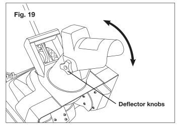
**WARNING!** Make sure that the chute deflector locks completely onto the discharge chute. An opening between the discharge chute and the chute deflector may allow foreign objects to be picked up by the snow blower and thrown in the direction of the operator causing serious bodily injury.
