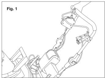
**2.** Secure the connection of the middle handle assembly to the upper handle by fastening the handle locks on each side (Fig. 2).
