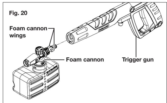
5. Turn on the pressure washer. Pull the trigger to operate the unit. The liquid detergent will automatically mix with water and be discharged through the nozzle.
