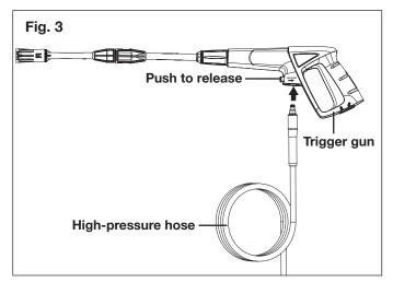
2. Connect the other end of the high-pressure hose to the water outlet on the pressure washer (Fig. 4). First, push the high-pressure hose end completely onto the high-pressure water outlet, then screw it on clockwise.
