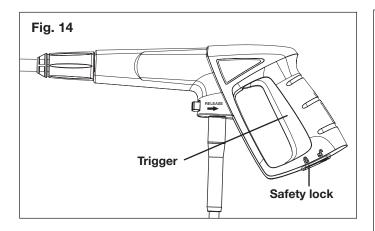
5. Keeping the trigger pressed, turn the switch to the ON (I) position to start the pressure washer (Fig. 15).
