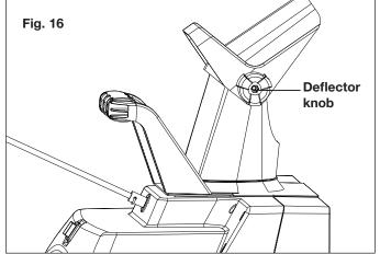
**WARNING!** Make sure that the chute deflector snaps and locks completely onto the discharge chute. An opening between the discharge chute and the chute deflector may allow foreign objects to be picked up by the snow thrower and thrown in the direction of the operator causing serious boldly injury.
