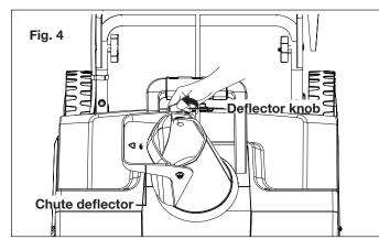
2. Secure the chute deflector by locking the deflector knob (Fig. 5).
