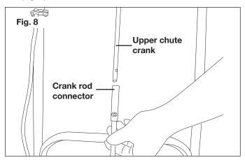
**4.** Align the screw holes and tighten the thumbscrew by hand (Fig. 9).
