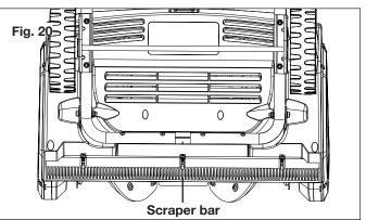
**2.** Detach the worn scraper bar from the snow thrower by removing the 3 screws that hold it in place (Fig. 21).
