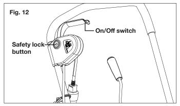
**3.** To power off, release your grip on the ON/OFF switch lever.
